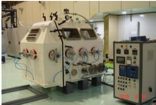
Welding Glove-box for Cavity Dressing
