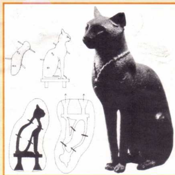
Stages of lost-wax ( cire perdue ) technique of hollow casting
