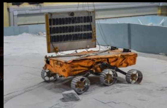
A model of the Chandrayaan 2 rover being tested at ISRO's simulated lunar soil facility. Credit: ISRO Chandrayaan-3's high-resolution camera will capture stunning images of the moon's surface,
