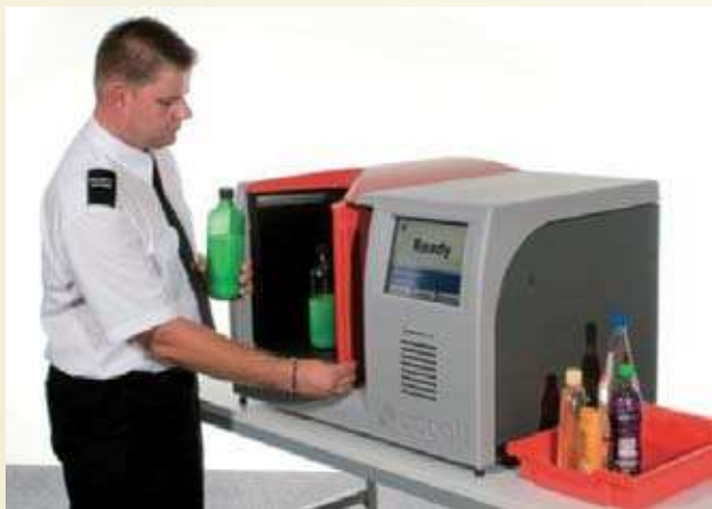
A scanner using spatially offset Raman spectroscopy can reveal the contents of packaged items that may conceal explosives or drugs (Credit: Cobalt Light Systems)
