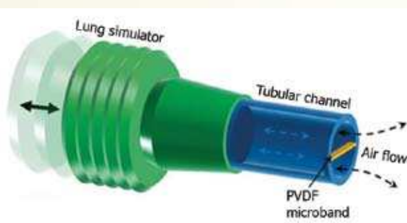
A simulated lung with the piezoelectric PVDF microband that vibrates as air flows past it (Image credit: EES Blog)
