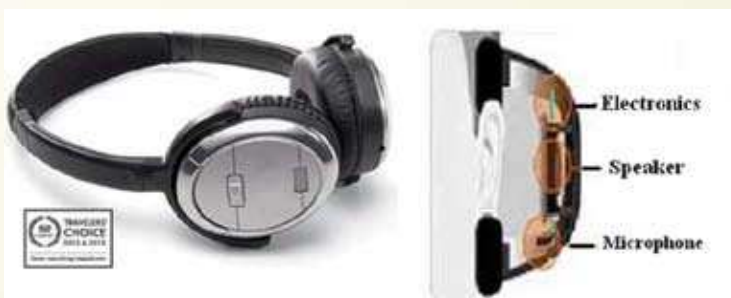
Acoustic noise cancellation head phone and its inside view
