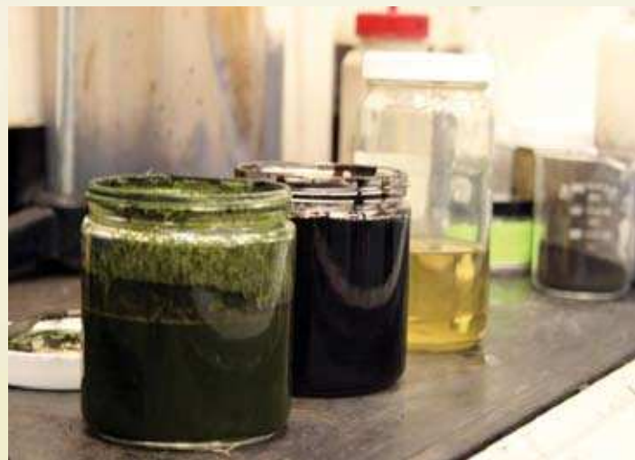
Steps in the process for making fuel from algae (from left): the algae slurry, crude oil, and refined diesel fuel.
