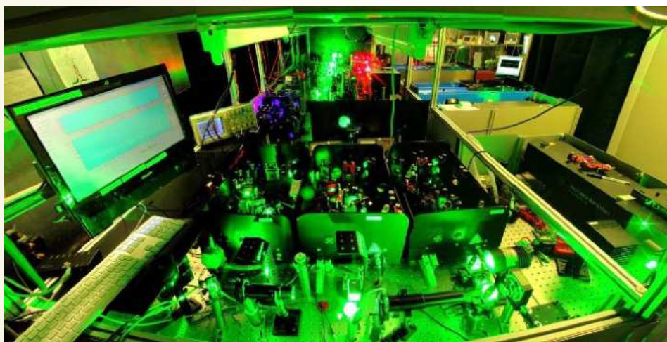
The Resonance Ionisation Laser Ion Source helps ionise rare elements like astatine at the ISOLDE facility. (Credit: University of York)
