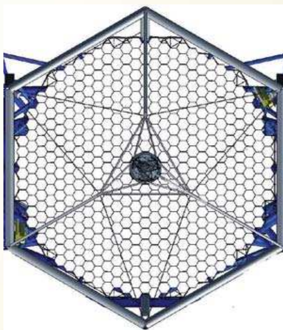
Sketch of the 30-m diameter primary mirror made of 492 hexagonal segments.
