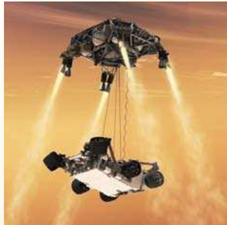
The final stage in the landing of Curiosity using a sky crane.
