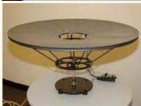
Deployment of antenna through shape memory property. Antenna in skewed form (top) Antenna in unfurled form (bottom)
