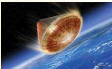
Atmosphere re-entering satellite protected by polymer ablatives
