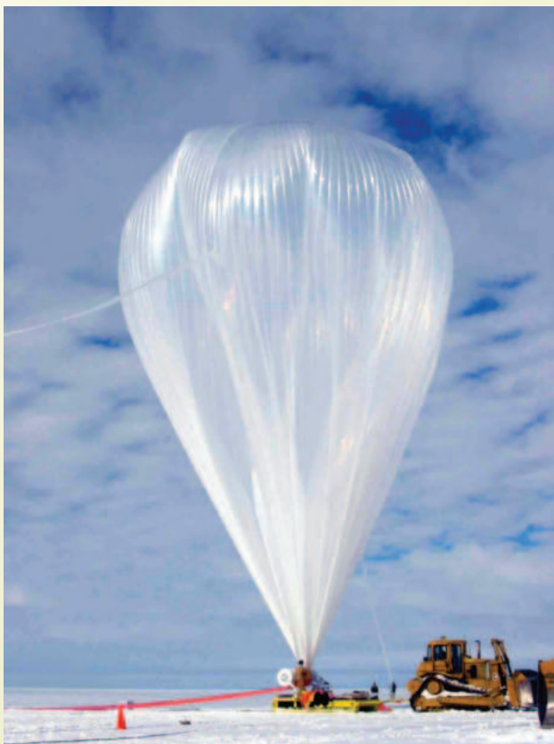
Balloon-borne ATIC detector being readied for launch in Antarctica (Photo: Seth White).
