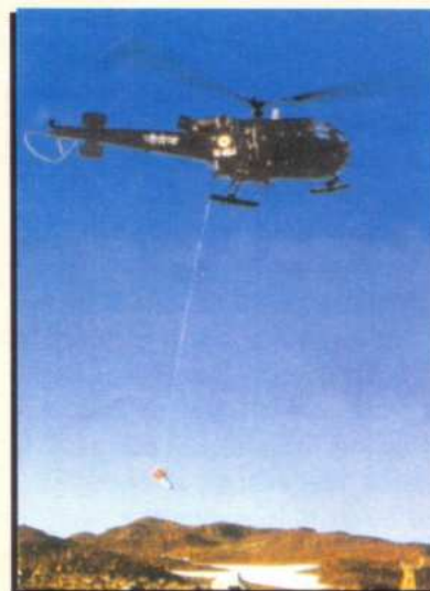
Helicopter-borne magnetic survey at Antarctica
