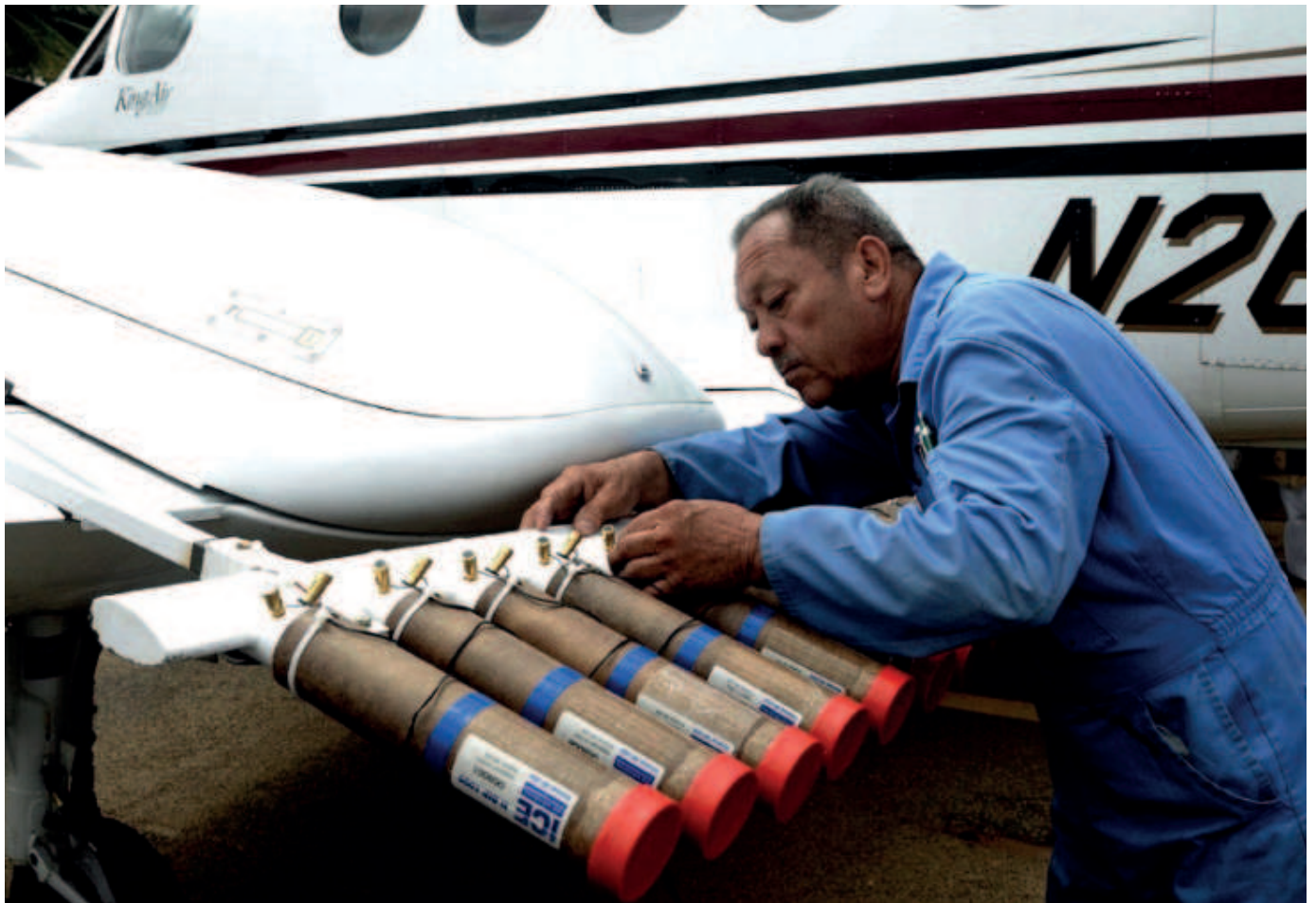
A technician fits canisters containing silver iodide, sodium chloride and potassium chloride onto a small aircraft for cloud-Seeding (Source: https://www.aljazeera.com )
