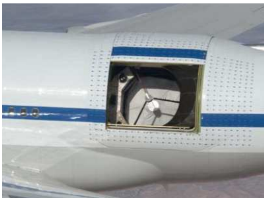
NASA's Stratospheric Observatory for Infrared Astronomy, SOFIA, carrying a 2.7-metre telescope, with open telescope doors.
