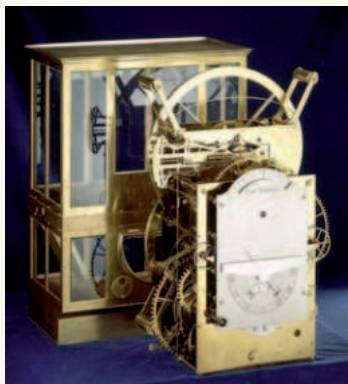
H3, Harrison spent nineteen years (1740-1759) working on this immensely complex timekeeper. For many years he was convinced it would win him the longitude prize
