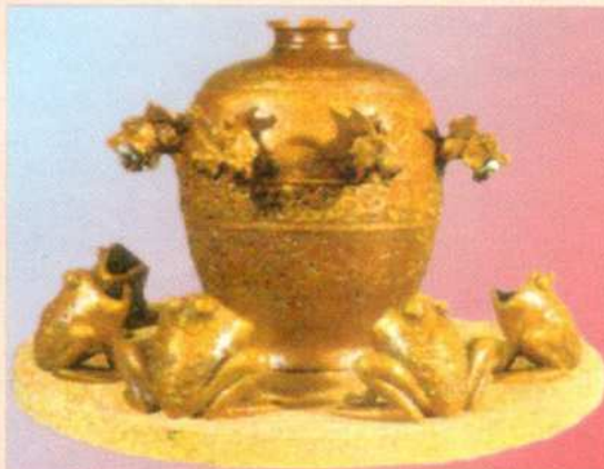
The earliest seismoscope invented by Chinese philosopher Chang Heng in A.D. 132
