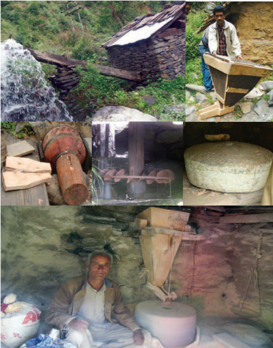
Figure 1: Various components of gharat and milling in progress. (a) Flume that diverts water on to the blades. (b) Hopper or a grain feeder that feeds grains for grinding. (c) Runner has blades, made of wood or iron, fitted to it. (d) The mill stone, rotation of which grinds the grain. (e) A happy miller and milling in progress. (Photo credits: 1a and e Alpy Sharma. All others: Sanjay Kr. Uniyal)
