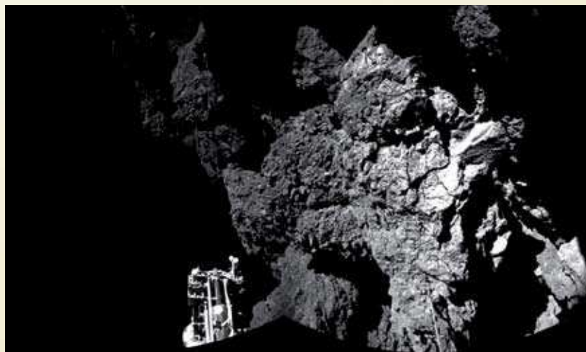
Philae after landing on the surface of Comet 67P/Churyumov-Gerasimenko. But the probe landed in a place where its solar panels could not recharge its battery. One of the lander's three feet can be seen in the foreground. (Credit: ESA/Rosetta Philae/CIVA)
