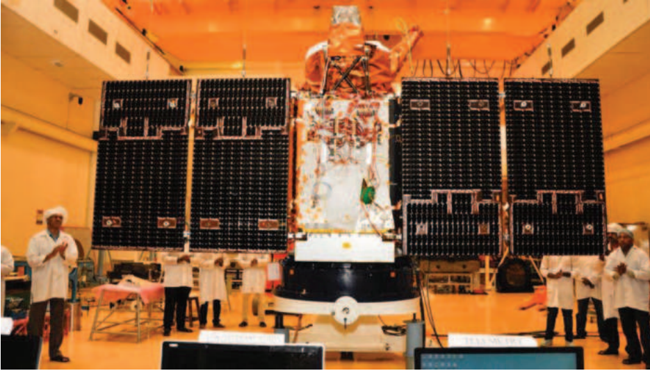
Fig.2. Cartosat-2 Series Satellite undergoing Panel Deployment Test (Credit: ISRO)
