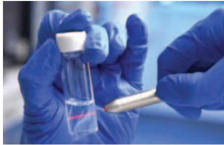
Laser beam can be seen scattered by nanoparticles in a solution of the UTSW-developed nanovaccine. (Credit: UT Southwestern)
