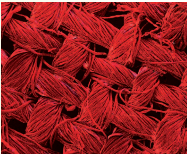
The red colour indicates the presence of silver nanoparticles – the total coverage on the image shows the nanostructures grown by the RMIT team are present throughout the textile. (Credit: RMIT University)
