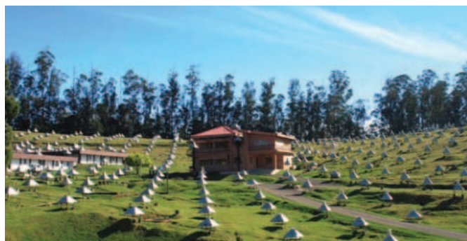
The GRAPES-3 experiment is a special telescope-array established in Ooty to detect muons from cosmic ray showers.
