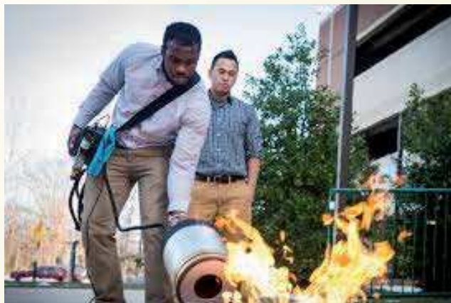
Seth Robertson and Viet Tran with their sonic fire extinguisher (Credit: Evan Cantwell)
