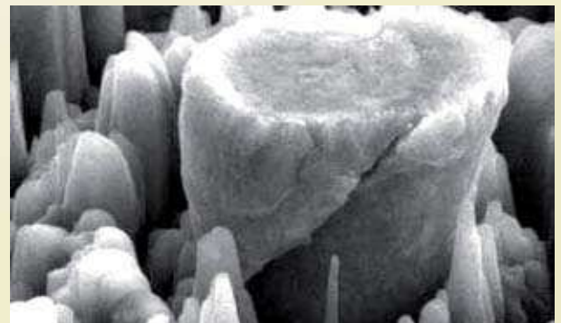
Electron micrograph of new strong metal made of magnesium with silicon carbide nanoparticles. (Credit: UCLA Scifacturing Laboratory)
