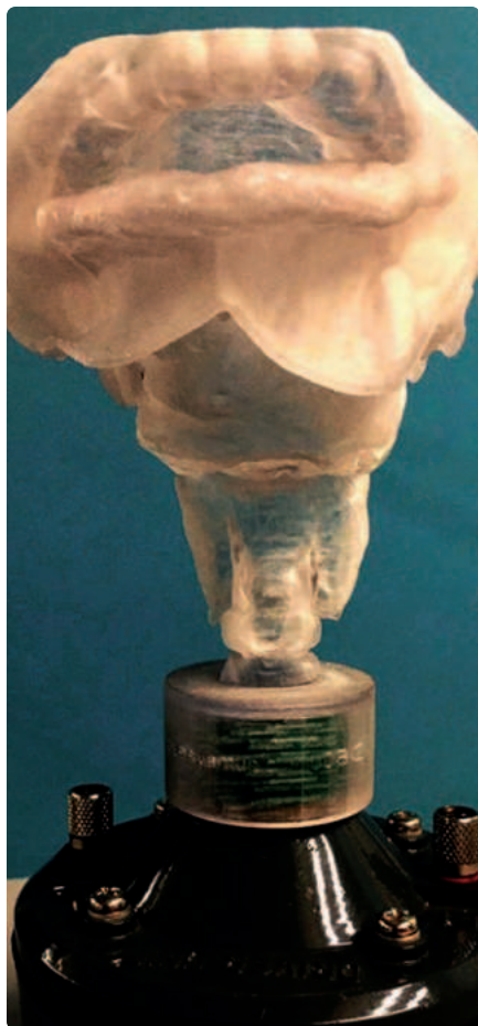
3D-printed vocal tract of the mummified body of Nesyamun. (Credit: David Howard)
