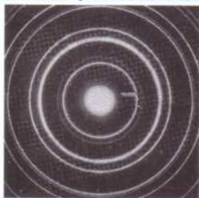
Left : Scattering of electrons by gold crystals Right : Scattering of X-rays by zirconium oxide crystals
