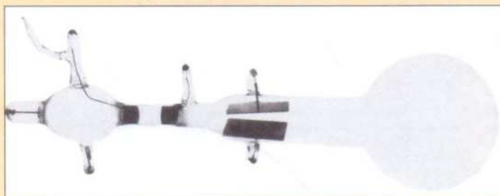
Fig-2 : Thomson's Tube for demonstrating that cathode rays are deflected by an electric field. It was also used to measure e/m .
