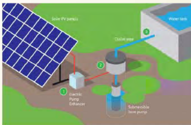
Solar water pumping system for irrigation
