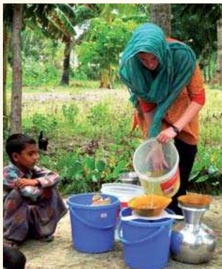
Dankovich pours contaminated pond water into a funnel containing an antimicrobial filter paper from “drinkable book” to obtain clean drinking water in a rural area of Bangladesh. (Credit: Ali Wilson)
