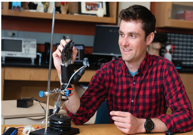
Electronic skin lets any prosthesis feel touch and pain. The skin is made of a combination of fabric and rubber, into which the electronic sensors are embedded. (Credit: img.newatlas.com)
