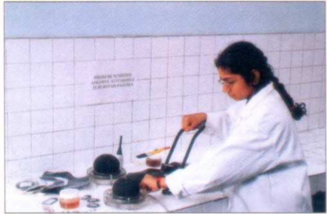
A pressure sensitive adhesive for instant repair of automobile tubes and tyres undergoing trials at the institute's laboratory
