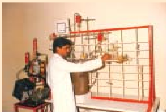
Preparation line at NRL for determining the oxygenating isotopic composition in water and plant tissues
